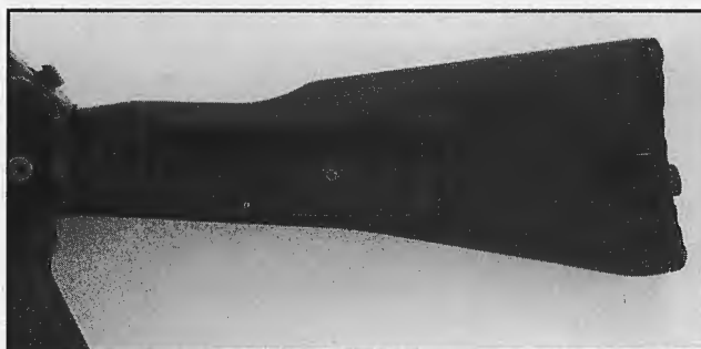
Left side of AK100 series buttstock, which is made from black, fiberglass-reinforced polyamide. Note cutout to accommodate scope mount riveted to the receiver and the spring-loaded latch at the rear which holds the side-folding stock against the left side of the receiver.
